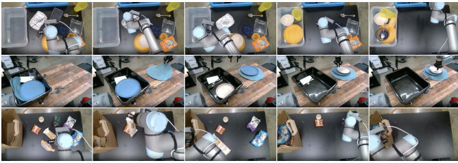
Fig. 8: The tasks in our language evaluation. We evaluate our model on 3 different language-conditioned tasks, each of which requires following a sequence of intermediate language commands. The tasks involve bussing a table (top) to put dishes in a bin and garbage in a trash bin, setting a table (middle) by taking items out of a bin, and packing a shopping bag (bottom).
